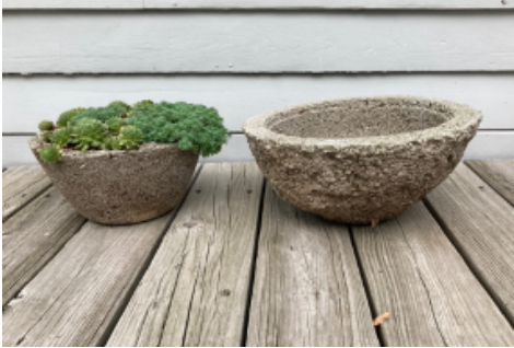
TROUGH ON LEFT WAS MADE BY PRESSING THE MIX ON THE INSIDE SURFACE OF A BOWL FORM RESULTING IN A SMOOTH OUTER SURFACE.
